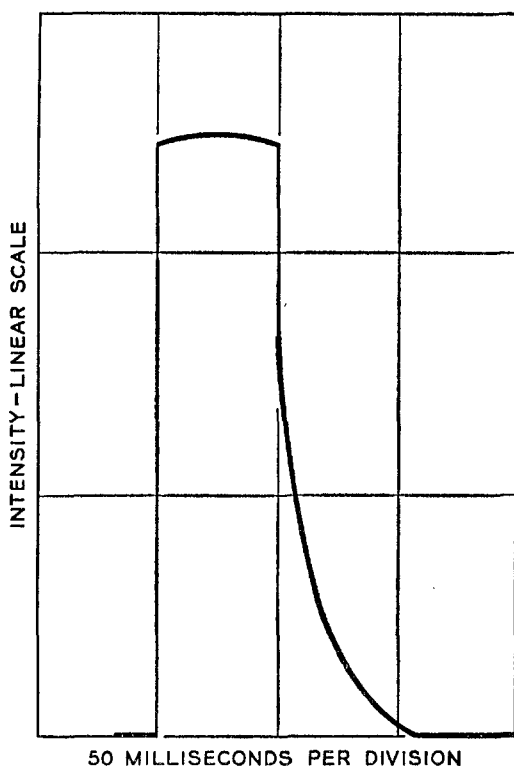
FIG. 1. A 50-millisecond light flash, such as was used in most of the experiments. (Redrawn from a photograph of an oscilloscope trace)
